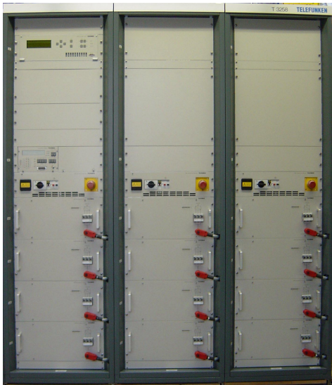
30kW solid state VHF/FM transmitter
